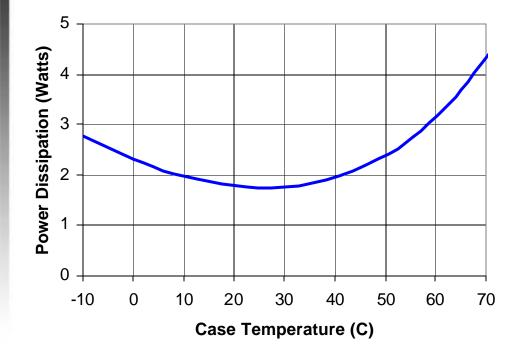
Measured Power Dissipation for 20 mW output at Vcc = 3.3V is:
