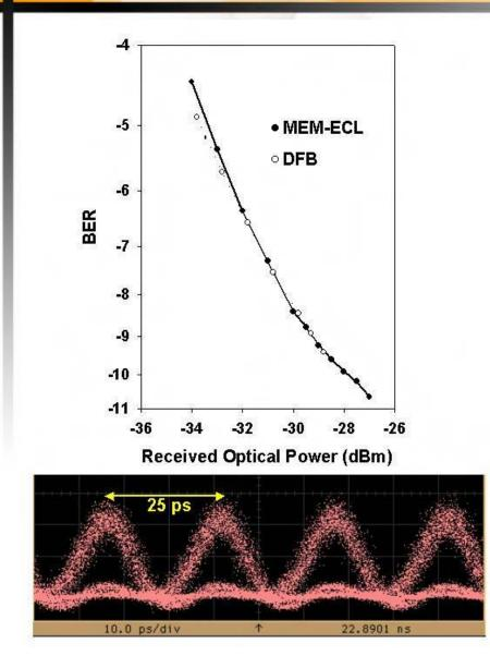
Nearly identical BER and transmitted eye diagrams in a 500 km amplified link at 40 Gb/s
